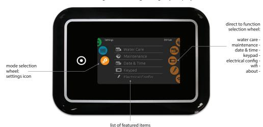
To select the settings mode, slide the left wheel up or down until the settings icon menu is highlighted in the middle.
